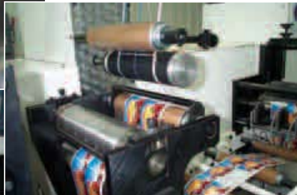
Left: print unit featuring quick set-up SAPS system (see box below), below left: Metronome press, below: Auto Peel-off allows waste stripping to start automatically
