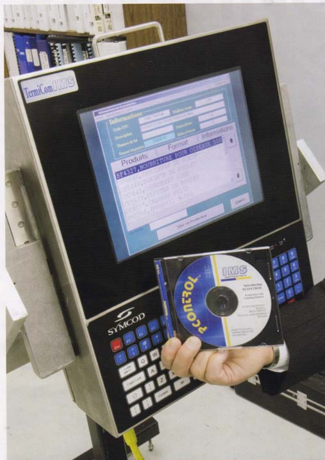
The IMS P-Control program is one of several recently-developed computer systems designed to ensure full product traceability for manufacturers.
