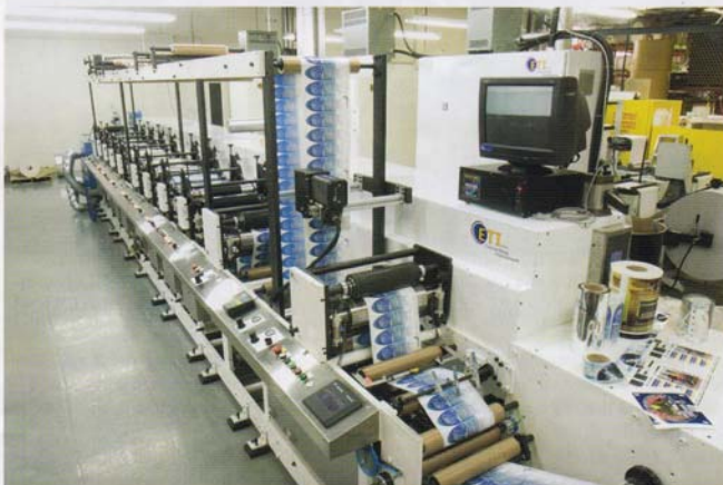
The recently-installed Metronome flexographic label printing press can handle print widths of up to 16 inches, at operating speeds up to 50 feet per minute.
