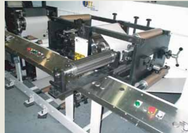
Sliding and accessible tools for faster changeovers
