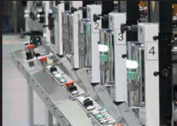
Printing stations with registration light indicators
